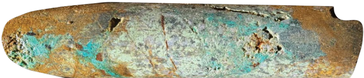
Figure 2. Malachite-Chrysocolla oxide assemblage overprinting mixed magmatic breccia (128.0-128.22 m; 1.71% Cu, 2.77 g/t Ag, sample G008434; KSMT25002)
